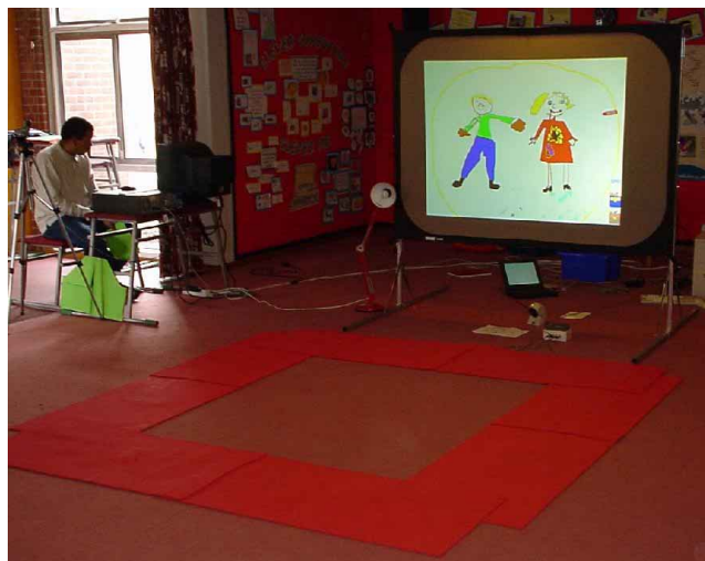
Figure 5: third prototype of the magic carpet with mats around the outside edge only (see color plate on page 557)
