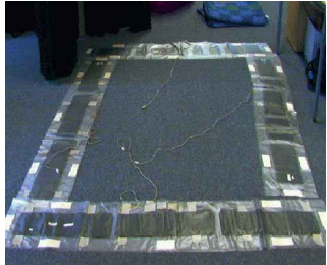
Figure 4: the design of the sensor pads for the third prototype magic carpet (see color plate on page 557)
