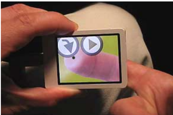
Figure 4: The nanoTouch device offers a 2.4" screen. A dot-shaped pointer corresponds to the touch location on the back. (In the mode shown, the device facilitates discoverability by simulating transparency , see section "pseudo-transparency").
