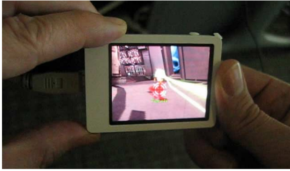
Figure 9: First person shooter running on nanoTouch through the prototyping environment (Unreal Tournament 2004)
