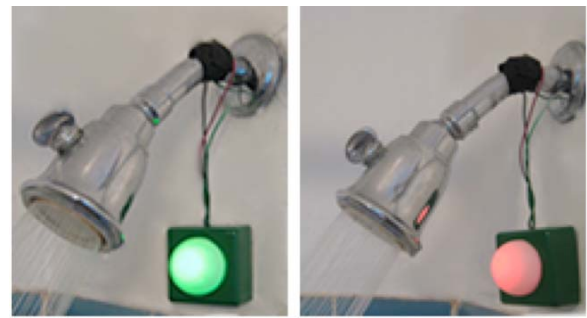
Figure 7. Ambient shower display mounted onto a shower in green state (left) and red state (right).
