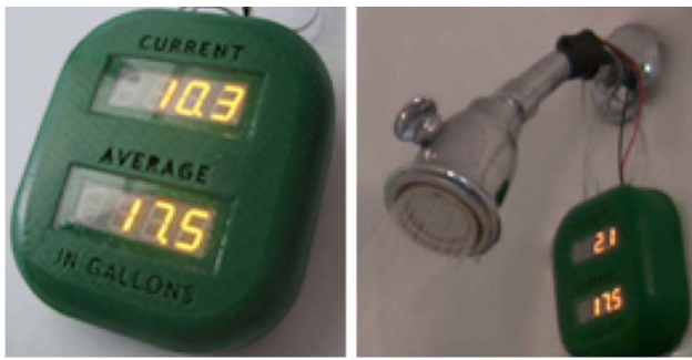
Figure 6. Numeric shower display showing current and average water usage (left) and installed in a shower (right).
