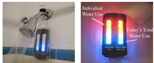
Figure 4. Pilot shower display mounted onto a shared semi-public shower (left) and labeled (right).
