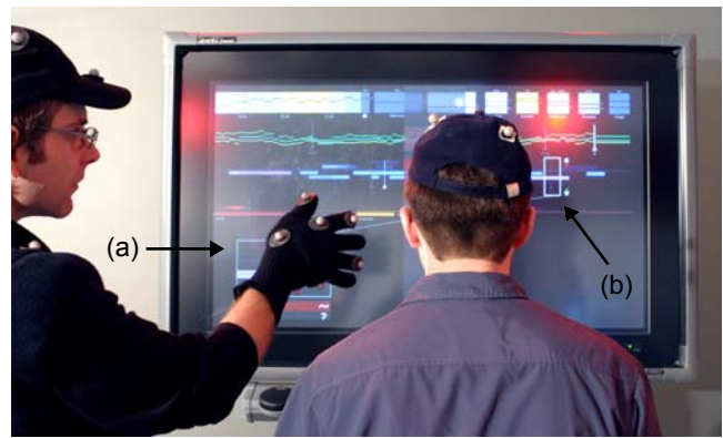
Figure 7. Using the reach gesture to access information beyond other users. (a) detail panel. (b) the selection point.
